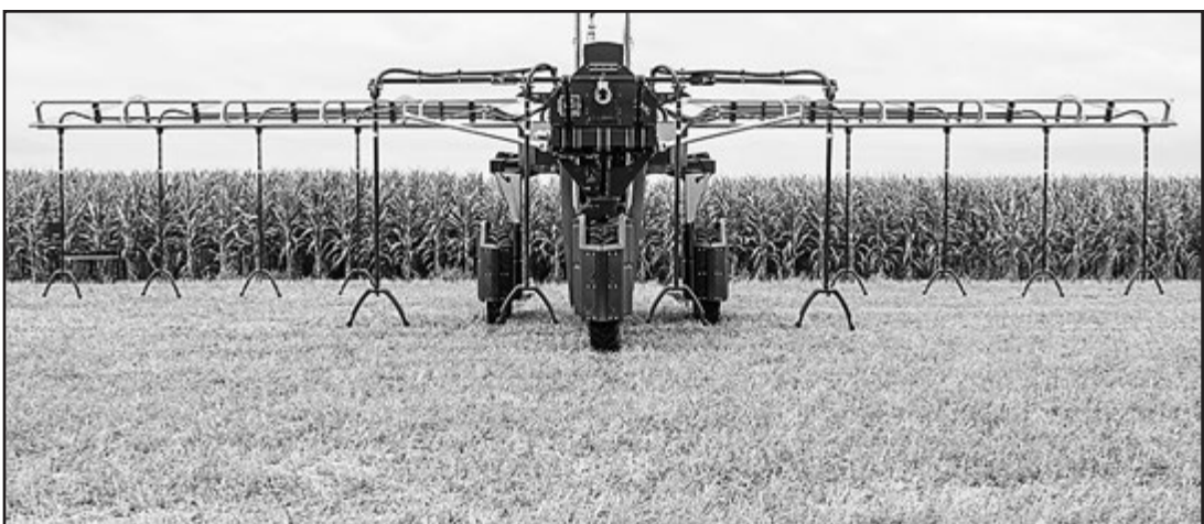
This highboy-type 360RAIN precision irrigator can also apply liquid manure, providing potential to expand the timing windows for manure application.
